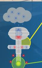
Controls and de-ionizes the electrical field with its multiple compensators neutralizing the formation of lightning in its protection area
