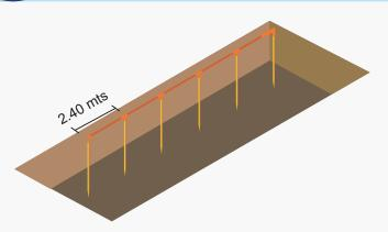
The separation distance between the electrodes must be equal to their length or twice as long as the determined area allows it. Example: If the electrode is 2.40mts, the distance between electrodes should be 2.40mts.
